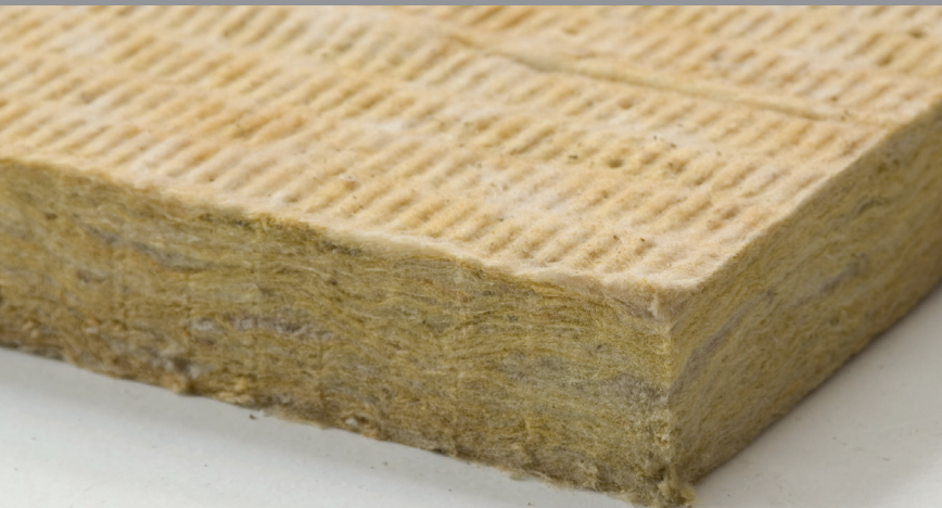
Industrial Board is a semi-rigid, preformed mineral fiber insulation that is suitable for temperatures up to 1200°F (650°C)
