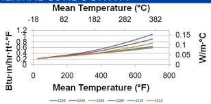
\*MinWool-1200 Industrial Board Insulation as tested in accordance with ASTM C518. THERMAL PERFORMANCE (IP UNITS) \*
